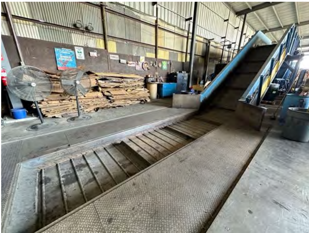
FIGURE 3: CONVEYOR BELT FOR COPPER SCRAP, GOING UP THE CONVEYOR BELT RAMP, BEHIND WHICH IS THE BAILING MACHINE
